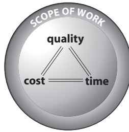
Figure 6.3 The time–cost–quality triangle. These three elements are interdependent for a given scope of work. Changing one element must have an effect on at least one other element, assuming the scope of work is unchanged
